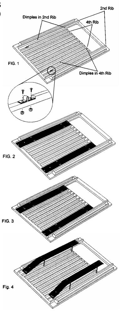
3) Position Skis as shown in Fig. 2. NOTE: Hole in end of ski should be at edge of shelter floor and angled end of ski is at edge of fishing hole. Insert ears of wire brackets into holes on one rib until the end of the ear hits the opposite wall of the rib. Then squeeze each wire bracket so you can insert other ear into hole in opposite rib.
