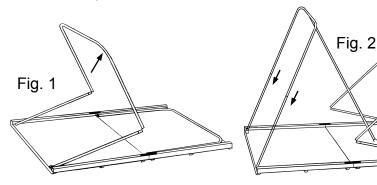
**4)** Fig. 2, Raise second U Frame, again keeping Frame about 24" away from Corners of Fabric Top. Assemble Frame and push into Corners of Fabric Top and adjust Seam in Fabric to follow Curve of the Frame. Clip end of Roof Tube Assembly to U Frame and slide next to inside edge of nuts as shown in Fig. 3 & 4. Clip second Roof Tube Assembly into place next to Nuts. With both Roof Tubes next to inside edge of Nuts...Install Roof Bows, Fig. 4.
