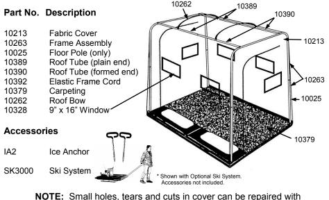
black duct tape applied to coated side of fabric.
